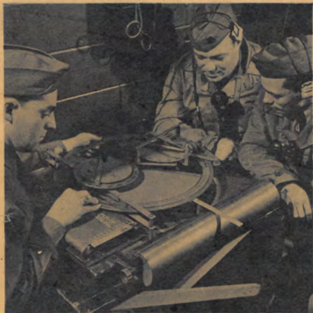
DEFLECTION BOARD is used in correcting aim for drift, windage. Each regiment has a weather crew.
