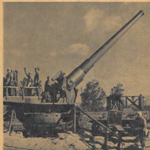
SIDE VIEW of this railroad gun shows how high its barrel must be elevated for all long-range shooting.
