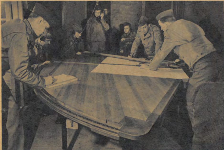
PLOTTING BOARD , housed in plotting car, is used to calculate direction, range of gun. Location of the target is charted from the lookout towers' telephone data.
